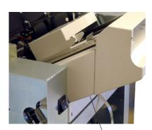
Adjustment screw below infeed module.
